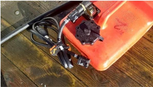
(2) This fuel line is **COILED**. In contrast to the squishy image to the left, this one is elegantly formed. Small coil with the cuff close to the tank.
